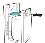
While pressing the switch inwards, push in the blue tab If the backplate is powered, the switch will flash or green If switch does not flash green, move to the next location & repeat step 1
